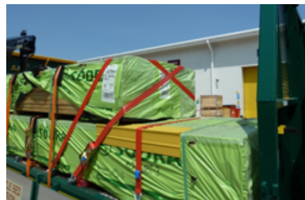
Figure 1: Full Loop Lashing
